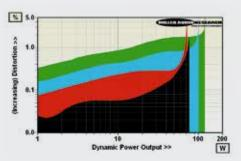
ABOVE: Dynamic power versus distortion into 80hm (black trace), 40hm (red), 20hm (cyan) and 10hm (green) speaker loads. Maximum current is 10.7A
